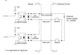
The input circuits of interface blocks of the product are illustrated in the figure above.
