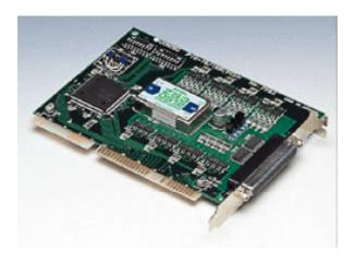
The PIO-16/16B(PC)H is a 16-channel digital input and output interface board for the IBM PC/AT and compatible computers. It can also be installed into a CONTEC I/O expansion unit. Plugged in a ISA bus expansion slot on the motherboard of a personal computer, can input and output up to 16 channels.
