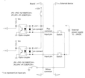
The input circuits of interface blocks of the product are illustrated in the figure above.
