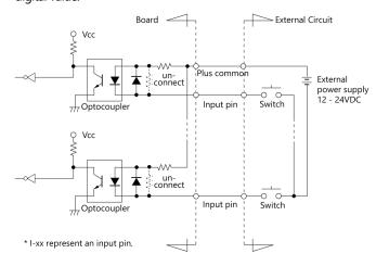
The input circuits of interface blocks of the product are illustrated in the figure above.
