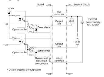
The output circuits of interface blocks of the product are illustrated in the figure above.
