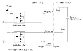
The signal outputs are solid-state relay outputs using a rated output current of up to 100 mA per channel.
