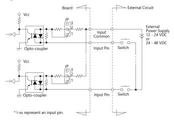
For each input channel, use the corresponding jumper to select a voltage range of 12 - 24 or 24 - 48 VDC depending on the voltage of the input signal.
