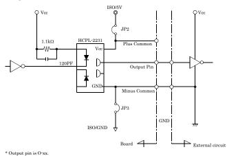
The output circuits of interface blocks of the PIO-16/16TB(PCI)H are illustrated in the image above. The signal output section is an opto-coupler isolated, TTL level output. Driving the output section requires an additional power supply isolated from the PC system. The board offers you an on-board isolated 5VDC power supply in option.
