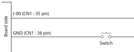
When the switch is ON, the corresponding bit contains 1.
