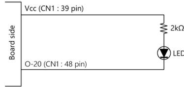
When "1" is output to a relevant bit, the corresponding LED comes on.
