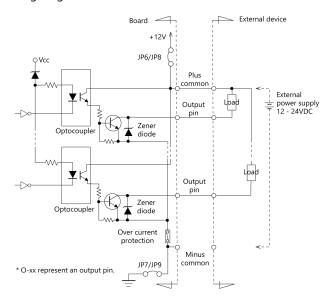
The signal output section is an opto-coupler isolated, open-collector output (current sink type).
