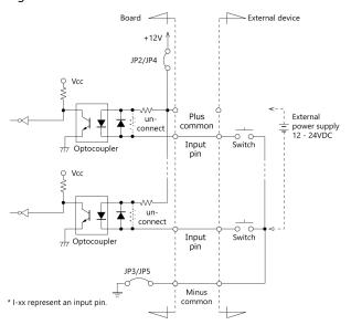
The signal inputs are isolated by opto-couplers (ready to accept current sinking output signals). This product therefore requires the on-board internal power supply or the external power supply to drive the input section of this product. The power requirement for each input pin is about 5.1 mA at 24 VDC (about 2.6 mA at 12 VDC).
