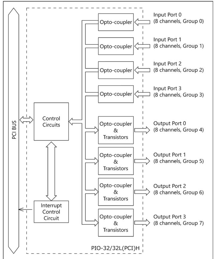
**Differences between the PIO-32/32L(PCI)H and PIO-32/32L(PCI)**
