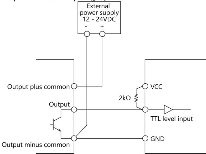
**Connecting the Sink Type Output and Sink Output Support Input**
