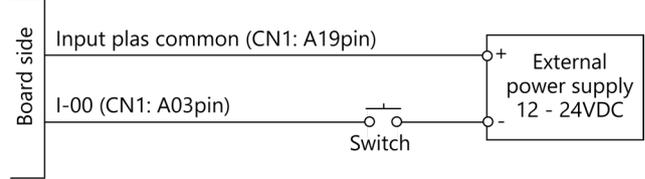
When the switch is ON, the corresponding bit contains 1. When the switch is OFF, by contrast, the bit contains 0.
