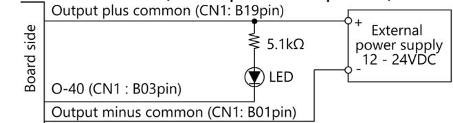
When "1" is output to a relevant bit, the corresponding LED comes on. When "0" is output to the bit, in contrast, the LED goes out.
