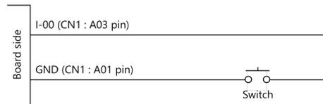
When the switch is ON, the corresponding bit contains 1.
