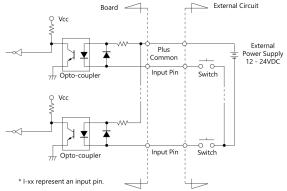
The input circuits of interface blocks of the PIO-64/64L(PCI)H are illustrated in the figure above.
