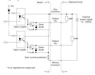
The output circuits of interface blocks of the PIO-64/64L(PCI)H are illustrated in the figure above.
