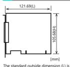
the distance from the end of the board to the outer surface of the slot cover.
