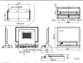
\*1: Make sure the tips of the screws do not intrude 5 mm or more from the plate surface. \*2: Make sure the tips of the screws do not intrude 8 mm or more from the plate surface.
