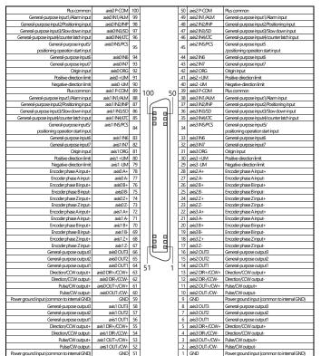
\* Axis0 - Axis3 of this manual corresponds to Axis No.1 - Axis No.4 in API-SMC(WDM).
