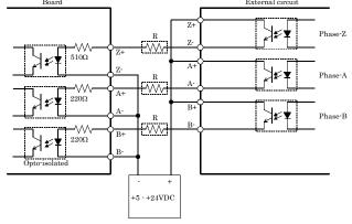
For open-collector output using an external power supply of +12 - +24 V, insert current-limiting resister R as shown in the diagram above. The R values are as follows. No R is required when +5 V is used.
