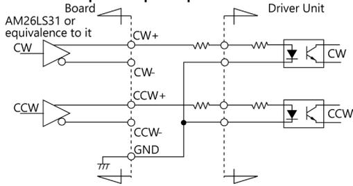
**Connection with TTL level input**
