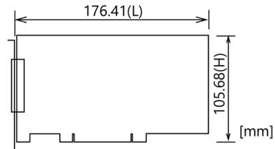
The standard outside dimension (L) is the distance from the end of the card to the outer surface of the slot cover.
