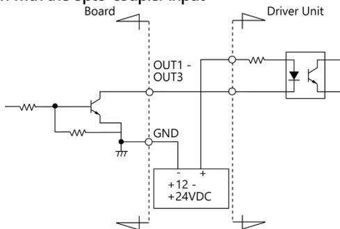
**Connection with TTL level input**
