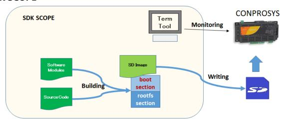
This SDK generates software modules in the cross-build development on the Host PC. If you wish to develop the software in the self-build development on CONPROSYS, please refer to the "Self-build" manual.
