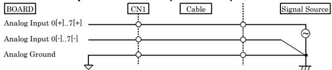
The following figure shows an example of 2-wire shielded cable connection. When the distance between the signal source and the board is long or you want to increase the noise tolerance, a shield cable connection is preferred. Each signal source is connected to a [+ ] pin of analog input channel and the signal common of this source to the [- ] pin of this input channel of CN1. In addition, the signal common must be connected to the pin of the analog ground of CN1 by the shielded braids.
