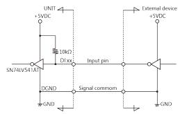
\*Input pins are indicated as DI xx. xx corresponds to input bits
