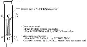
Pin Assignments of Interface Connector
