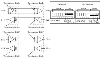
The figure below shows the circuit associated with the data transfer mode setting switch and terminator setting switch.
