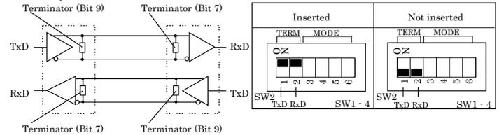
The figure below shows the circuit associated with the data transfer mode setting switch and terminator setting switch. Each channel shares the same switch and the bits to be set are vary.
