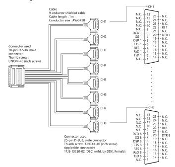
Connection conversion cable (Option) Connection Conversion Cable for RS-232C (78P→25P x 8, 1m)
