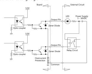
The signal output section is an opto-coupler isolated, open-collector output (current sink type). The rated output current per channel is 100mA at maximum. The output section can also be connected to a TTL level input as it uses a low-saturated transistor for output.
