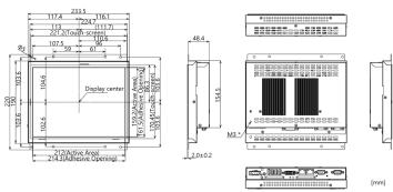
\* Keep the penetration length from the housing suface to the end of the M3 screw 9mm or less. Using longer screws can damage the internal components.
